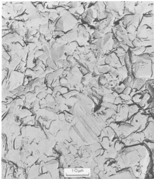
Figure 4 The blocky microstructure of mullite crystals after rapid formation following heat treatment at 850° C for 4 h and 1090° C for 4 h. Etched with 15% HF for 4 min at 23° C.
